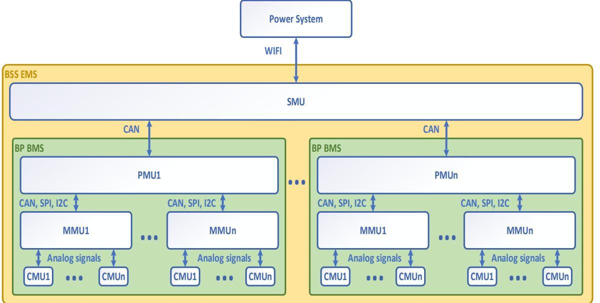
Figure 1 Communication between different nodes within battery packs and swapping station
