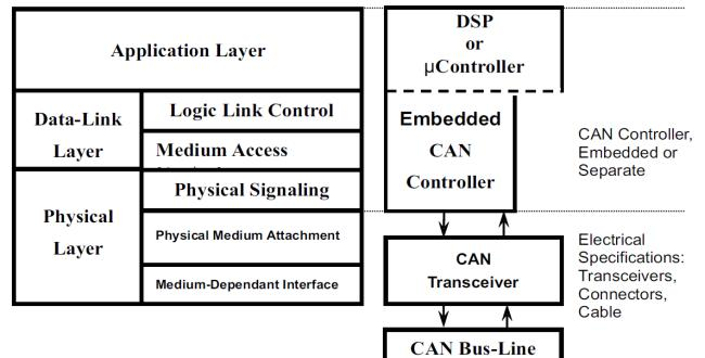
Figure 2 The Layered ISO 11898 Standard Architecture
